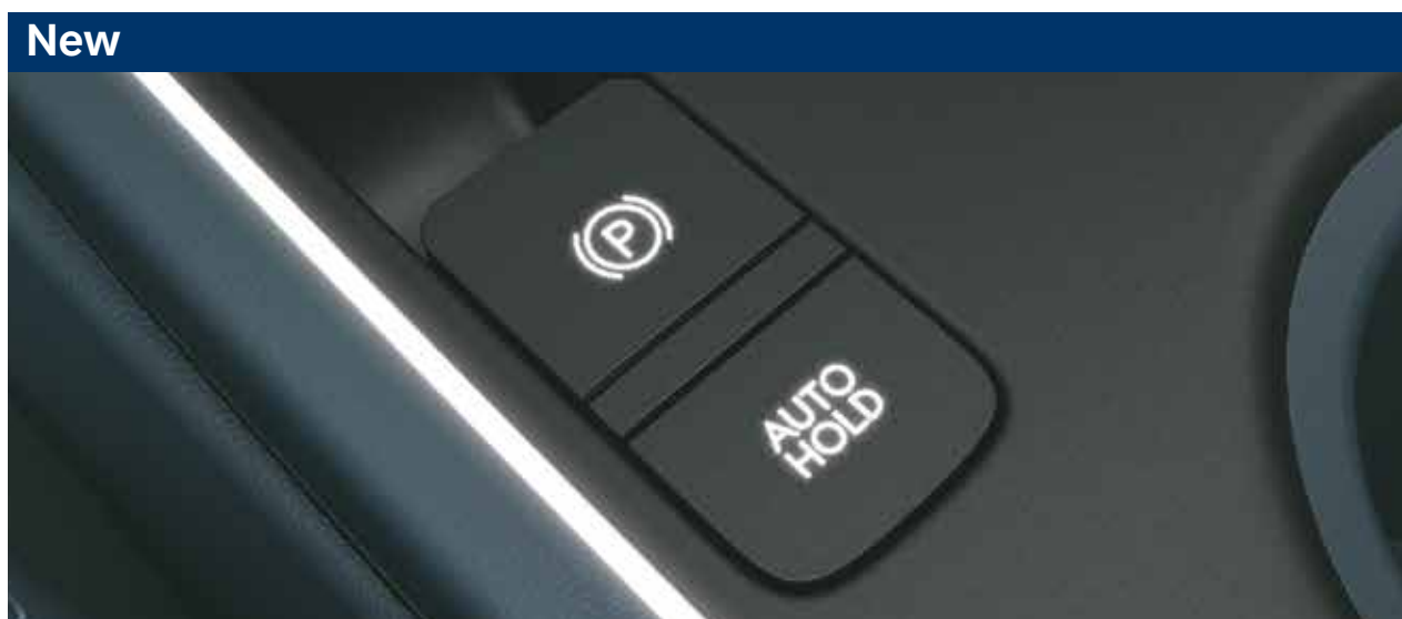
Electronic parking brake (EPB) with Auto hold
